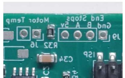
After connection, test to ensure that when the motor rotates in one direction, the limit switch corresponding to that direction stops the motor. If this is not the case, the End A and End B wires must be reversed.
